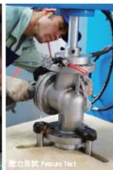
壓力測試 Pressure Test
